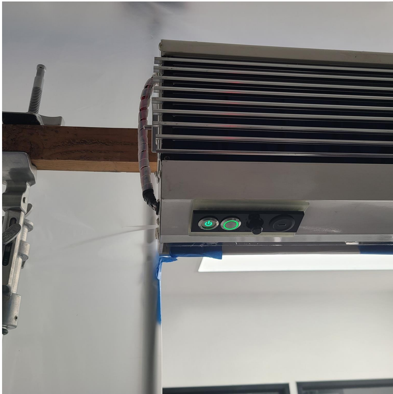
Figure 3. Visual light on Ion Bar indicating fan and ionizer on.
